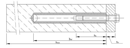
$t_{fix}$  = thickness of fixture
